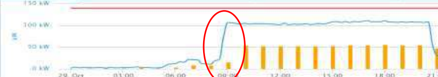
The chart shows the power consumption and the power demand are not matching. It indicates some equipment are powered-on in the same time.
